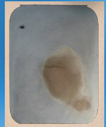
Exposure 20 [min] away from TNTL. In some cases plastic backing was spoiled!
