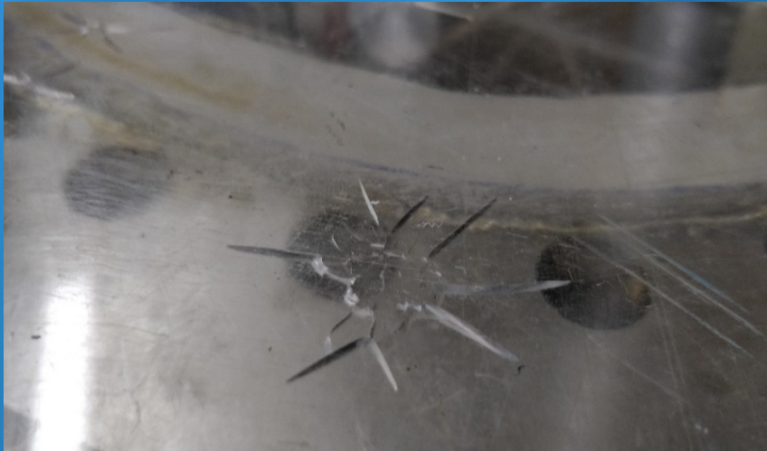
Left. Inside plexiglass 33 [mm] thick.
